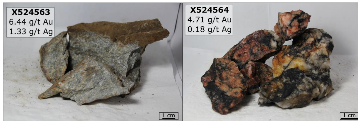
Figure 3. Images of grab samples X524563 and X524564, resulting in gold grades of 6.44 g/t Au and 4.71 g/t Au, respectively.
